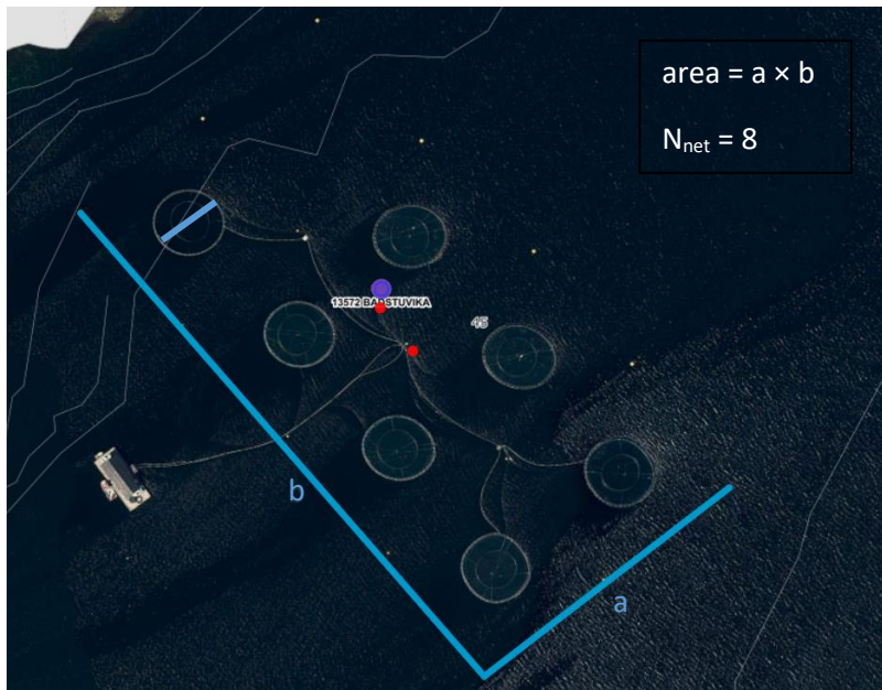
Figure 2. Example of data obtained from visual inspection of a site. The blue lines show the measurement of the diameter of the nets and the area (length and width) occupied by the nets. The mooring buoys, visible as white dots on the image, were used as outer points for the length/width measurements. The chosen value for number of nets, N_{net} , at each site was set to the number representing the production at full capacity. In this image, the area is thus a \times b (before adding the additional 150 m to length and width), and N_{net} is 8.
